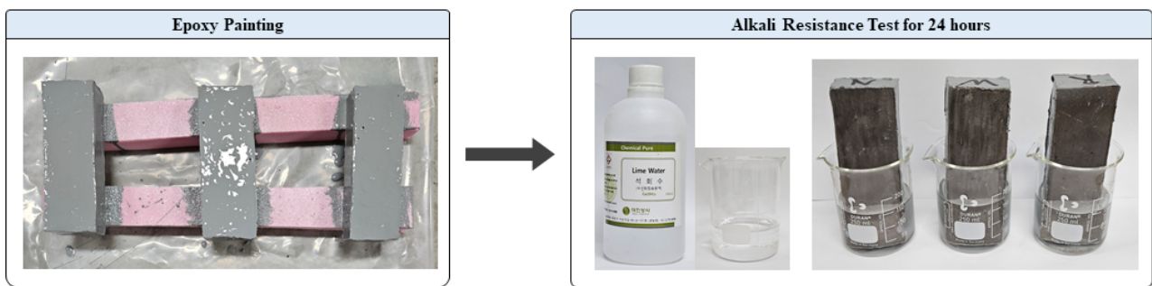
Figure 3. Alkali resistance test methodology
