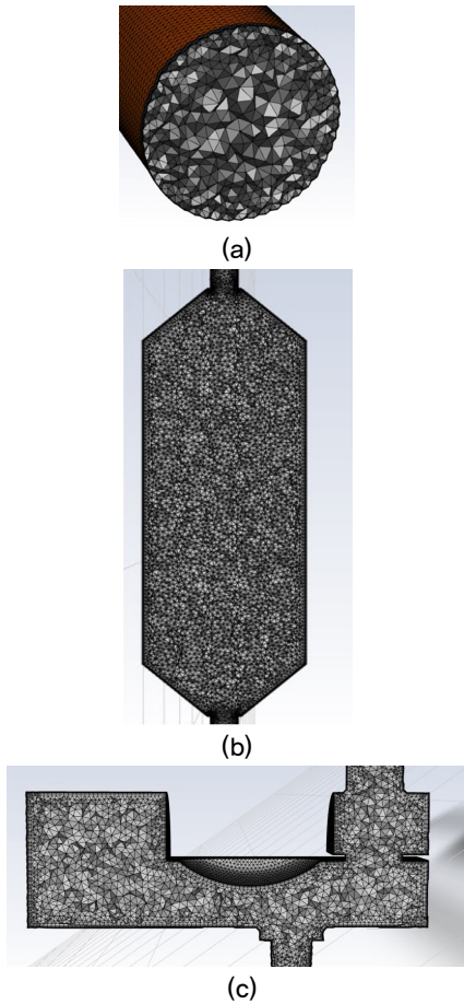
Fig. 2. (Color available online) Section view of mesh configuration at the (a) pipe, (b) muffler and (c) 4-way valve.
