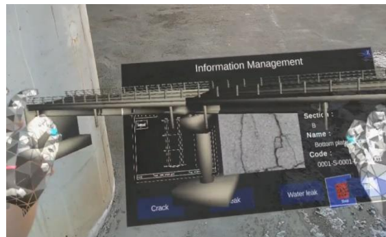
Figure 11. Left and Right Rotation/Extension of a BIM 3D Model on AD Display
