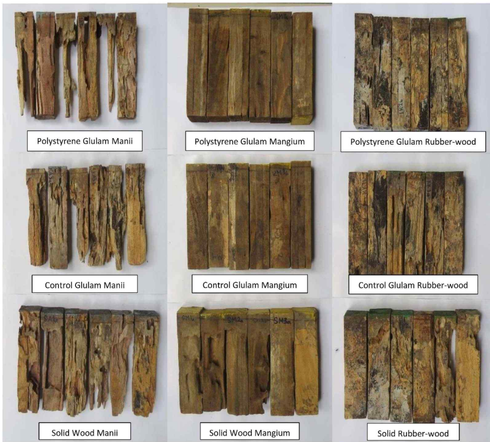
Fig. 6. Test sample after exposure in the field of each wood species and wood product.
