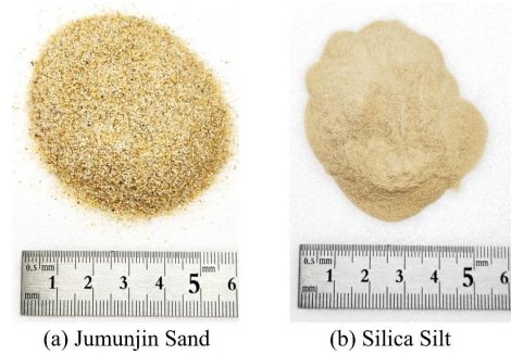
Fig. 1. Image of material used in this study: (a) Jumunjin Sand, and (b) Silica Silt
