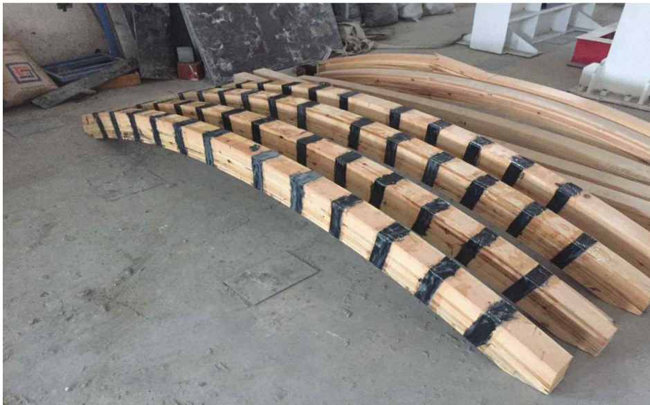
Fig. 4. Application of CFRP fabrics to arches as stirrups. LVDT: linear variable differential transformer, CFRP: carbon-fiber-reinforced polymer.
