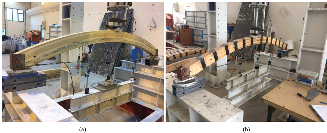
Fig. 6. Schematic view of the static load test set up. (a) Flexural loading system of reference sample. (b) Flexural strength tests of timber arch sample wrapped outside with FRP. FRP: fiber-reinforced polymer.
