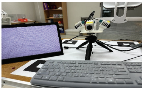
Fig. 3. Camera and marker pattern placement for calibration.
