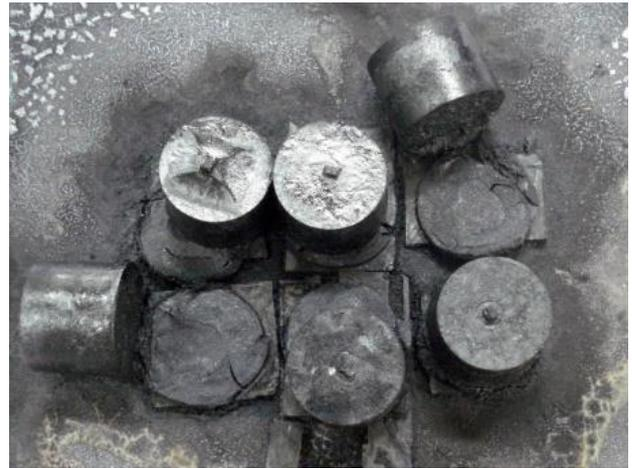
Fig. 10. Oxide superconductors prepared by a powder synthesis method (Diameter of the samples is 25 mm).
