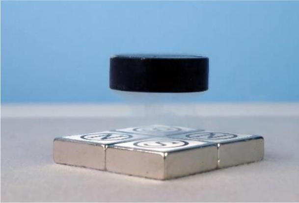
Fig. 12. Meissner effect of a YBCO superconductor (Diameter of the sample is 40 mm).
