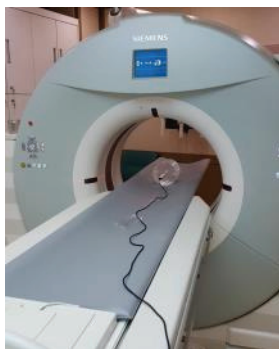
Fig. 1. CT scanning for dos calculation of CTDI head phantom.
