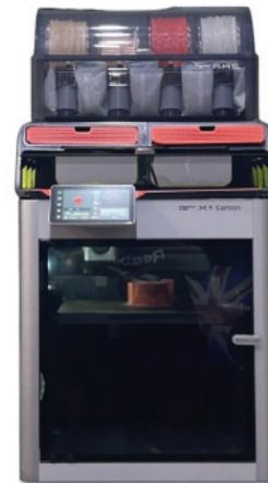
(b) Phantom output 3D printer of the FDM type
