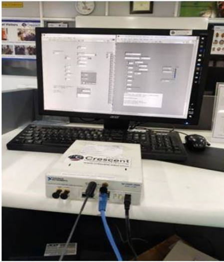
FIGURE 6 Experimental setup of the proposed QC-LDPC code, using USRP 2920
