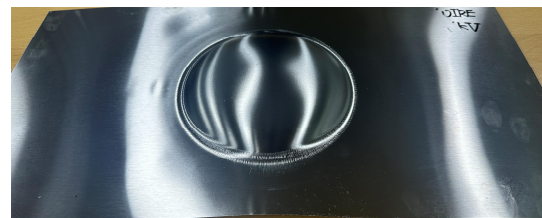
Fig. 8 Result of free bulging experiment with wire electrode at 6kV
