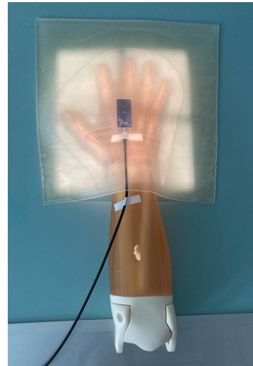
Fig. 1. Set-up detector covered by bolus for measuring entrance dose on the hand phantom.
