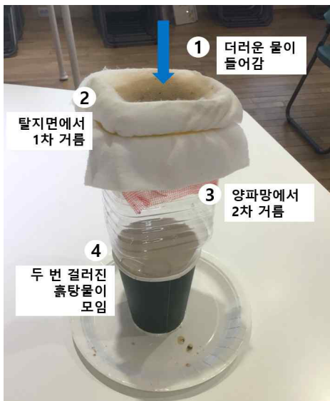
Fig. 4. Group B's final water collecting device using condensed cotton balls
