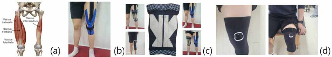
Figure 6. (a) Appearance of the Lower Extremity Anatomy, (b) Design Process via Kinesio Taping Technique, (c) Appearance of Completed EMS Knee Protector, (d) Appearance after EMS Module Assembly
