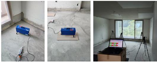
Fig. 4. (Color available online) Lightweight floor impact sound measurement on floor finishing materials in mock-up laboratory.
