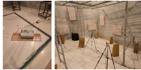
Fig. 2. (Color available online) Lightweight floor impact sound measurement in the D laboratory.
