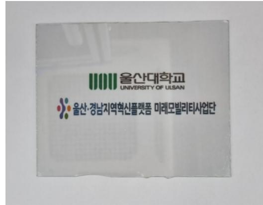
Fig. 1. The image of the ZnO 30 nm/Cu 10 nm/ZnO 30 nm thin film.
