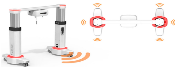
[Fig. 10] Active safe system of Patient Transfer Robot
