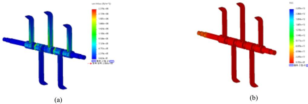
Fig. 12. Results of static analysis (Case 5). (a) is distribution of von-mises Stress. (b) is distribution of FOS (Factor of Safety).
