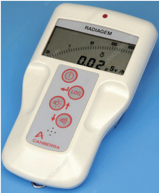
Fig. 2. Radiagem™ 2000 personal portable dose rate and survey meter.
