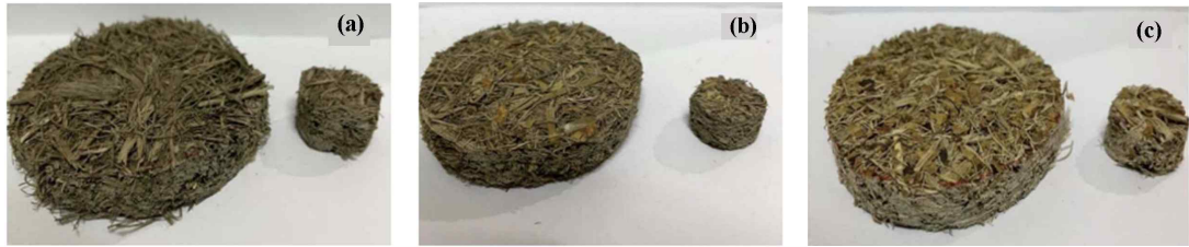
Fig. 2. Composite samples (a) SB100, (b) SB75-CS25, (c) SB50-CS50. SB: sugarcane bagasse, CS: coffee silver skin.
