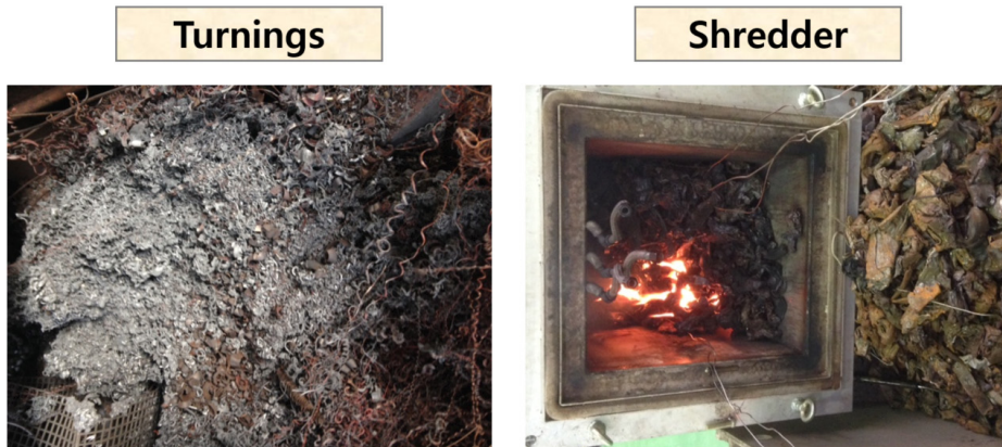
Fig. 4. Photographs of Turnings and Shredder after scrap preheating experiments.
