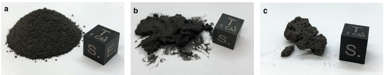
Fig. 6. Processing MGS-1 primary phases, (a) Mixed primary phases, including plagioclase, basaltic glass, pyroxene, olivine and magnetite, (b) Paste formed from primary phases, water, and sodium metasilicate, (c) Resulting solid cobble formed after the paste is dried and solidified
