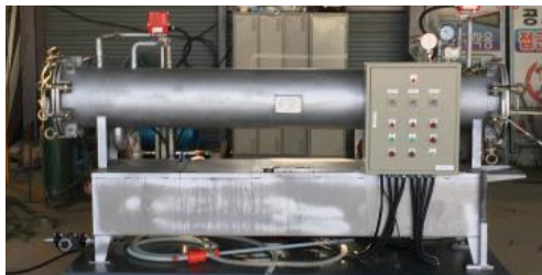
<Figure 2> Vacuum Pressure Impregnation Facility
