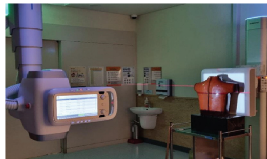
Fig. 1. The phantom was placed in front of the detector.
