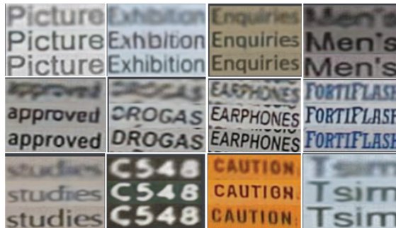
Fig. 9. Image visualization: images with the same character are represented as a group, and from top to bottom are LR text images, SR images generated by the proposed model, and HR text images.
