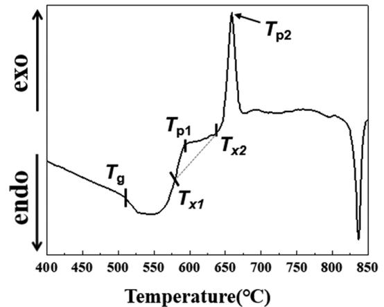
Fig. 2. DTA curve of 50B10L40BF glass.
