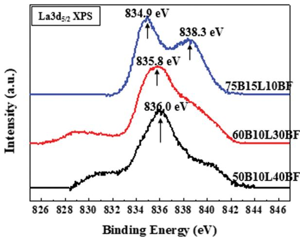
Fig. 5. Normalized  $\text{La}3d_{5/2}$  XPS spectra of glass samples.
