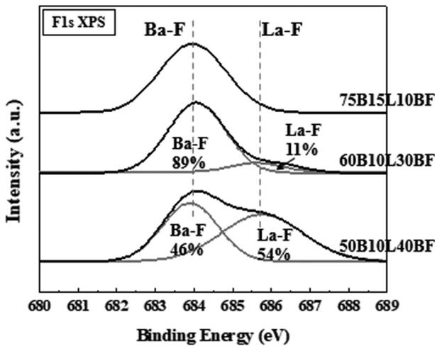
Fig. 7. Normalized F1s spectra of glass samples.
