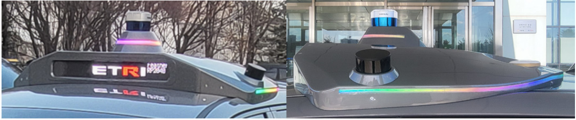
<Fig. 4> Autonomous Driving Vehicle situation information display UI design for frontal LED matrix(left) and multi stripe LED structure(right)
