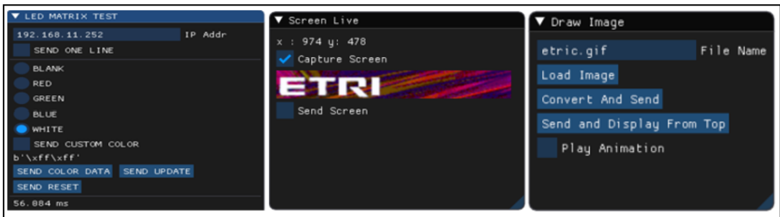
<Fig. 2> Multi-matrix LED main control client GUI(left), configuration of playing video(middle) and static image(right)
