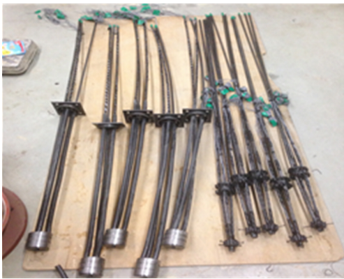
(a) Compression and tension type anchor
