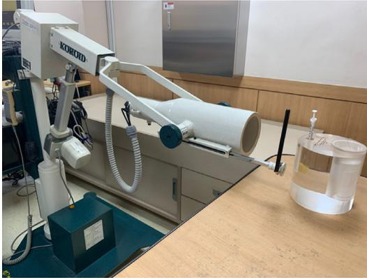
**Fig. 1.** Neck Phantom is designed to simulate a patient's neck. The phantom is constructed of lucite. It has a two part insert that allows counting from a bottle, vial or capsule. A capsule holder is supplied to enable the user to count capsules directly. The phantom's cylinder and carrier have scribelines for accurate alignment. A flat surface on the cylinder allows either vertical or horizontal positioning.
