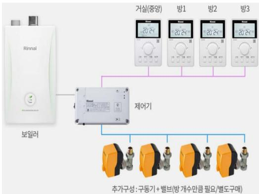
Fig. 8. Room Controller System Configuration Diagram[4]
