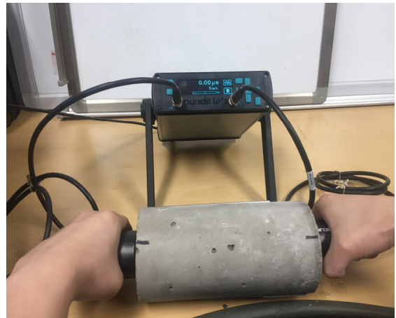
Fig. 3. Ultrasonic pulse velocity measurement
