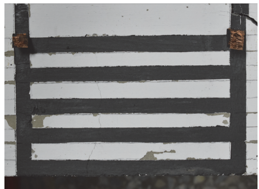
Fig. 12 Flexural crack in R5 pattern after testing
