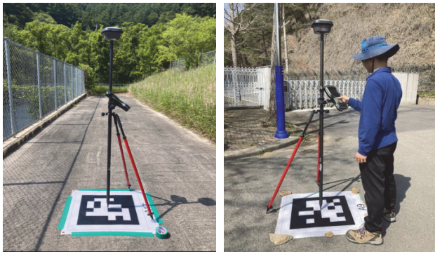
Fig. 1 April Tag as a GCP with surveying
