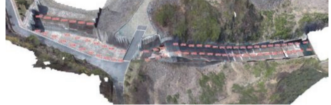
Fig. 7 Inspection Grid Map of JAR Dam Spillway
