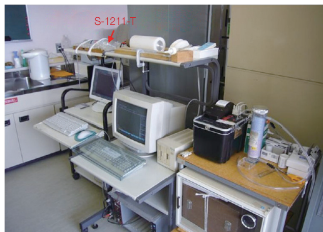
Fig. 2. A diameter of 76 mm and a length of 76 mm NaI(Tl) scintillation detector (S-1211-T, energy resolution of the detector in terms of FWHM is 7% for ^{137}\text{Cs} ; Teledyne Brown Engineering Environmental Services).
