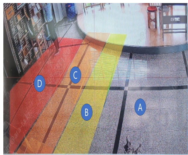
[Figure 8] The implemented system: (A) safe zone, (B) Warning zone, (C) Slow zone, (D) emergency zone
