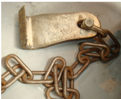
Fig. 5. Chain sling employed improper chain.
