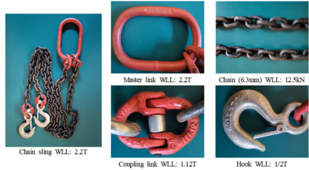
Fig. 4. Chain sling with different rated loads of components.
