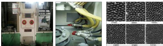
Fig. 10. Shot blast surface treatment and shot ball
