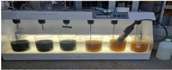
Figure 1: Comparison according to the amount of sodium hypochlorite injected (Exp 1)
