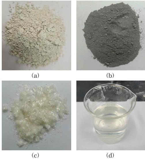
Figure 2. Materials used in this study: (a) Blast furnace slag, (b) Silica fume, (c) PVA fiber and (d) Alkali activator
