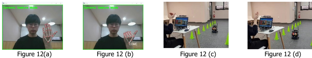
Figure 12. Hand dynamic mode gesture “COME” recognition and robot control
