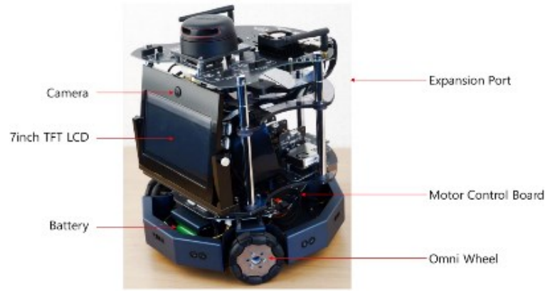
Figure 8. Experimental robot with 3 omni wheels
