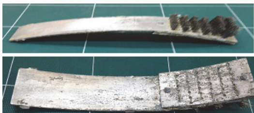
Fig. 6 Braided stationary wire brush parts (Reproduction)
