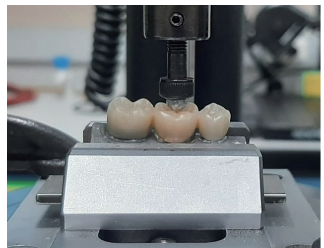
Fig. 3. Position of the 5 mm steel ball on the fixed dental prostheses.
