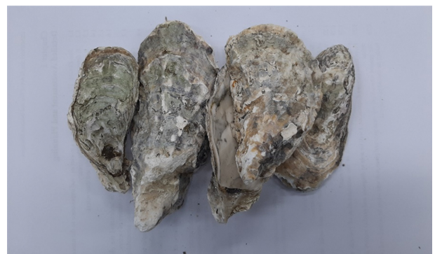
Fig. 1. Oyster waste shells used to prepare inorganic fillers.
