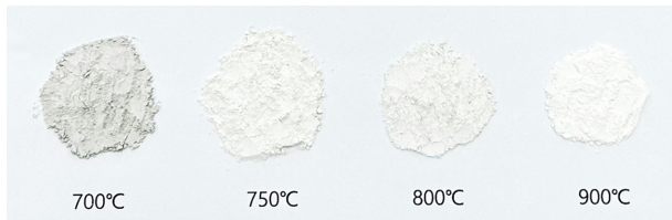
Fig. 6. Color change of the oyster shell powders heat treated at different temperatures from 700 to 900°C.
