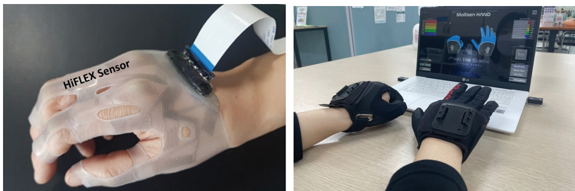
Fig. 2. ROM test with Mollisen HAND and soft sensors embedded in gloves.
