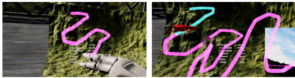
(a) Scanning path drawing (b) UAV's automatic flight Fig. 3. Defining SAR UAV flight path by hand gesture at the mountain site
