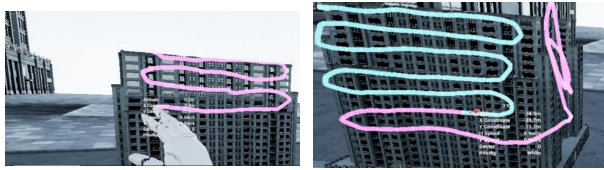
(a) Scanning path drawing (b) UAV's automatic flight Fig. 2. Defining SAR UAV flight path by hand gesture at the building site
