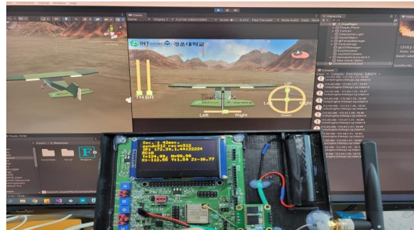
Fig. 11. Joystick combined with simulation via WiFi
