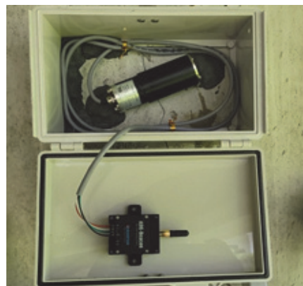
(b) Crack gauge
