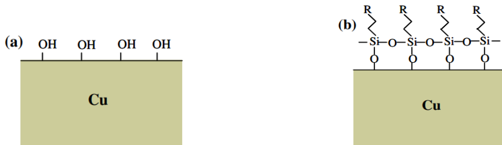
Figure 2. Surface chemistry diagrams of (a) untreated cu surface and (b) organo-functional silane-treated cu surface
