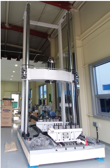
Figure 5. Fatigue testing apparatus and test specimen
