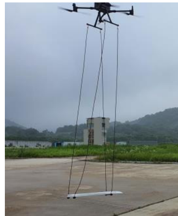
Fig. 1. Photo of MATRICE 300 RTK and MagArrow combined
